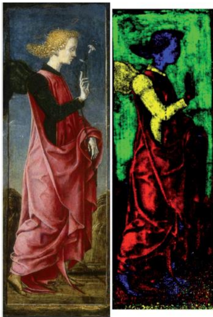
Fig. 4 Visible image and endmember map for Gabriel. (Left) Colour image. (Right) False-colour image showing the locations to which the endmembers map in the panel. Egg yolk binder (red EM) maps mainly to Gabriel's red robe. Glue binder (blue EM) maps to areas of the face and feet. Azurite in a glue binder (green EM) and malachite in an egg yolk binder (yellow EM) map to the sky and dark green tunic and wings, respectively.
